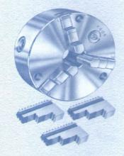
**Type AS-G:** SECO GOLD TRUGRIP self centring ACCURACY ADJUSTABLE chucks have a unique micro adjustment system which enables this chuck to achieve high concentric accuracy of .005mm and repetitive accuracy of .013mm. The AS-G type chucks come with forward and reverse sets of Jaws, dual purpose Operating Key and Mounting Bolts.
