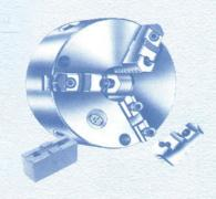
Type MTSJ3G: SECO GOLD 3Jaw self centring (TRUE) chuck is supplied with forward and reverse sets of Jaws, Operating Key Mounting Bolts, Allen key and an additional set of Master Base Jaws fitted with Top soft Jaws.
